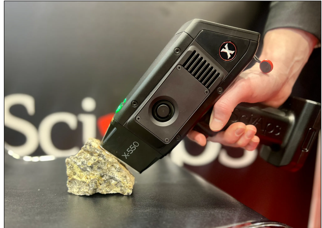
Example of elemental analysis by portable XRF (SciAps)
